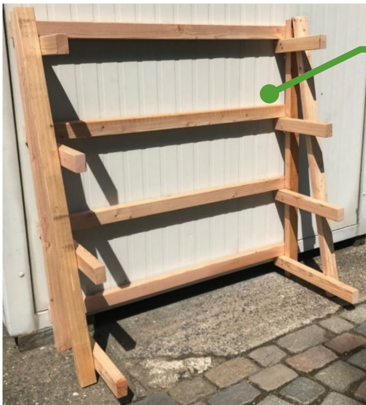
Figure 15: Adding the struts.
