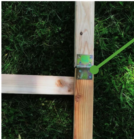
Figure 14: Assembling of the front frame using hinges – in detail.
